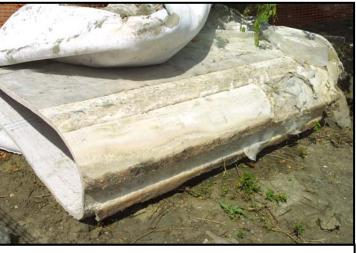
Photo 2 – Section of uncured fiberglass liner.
